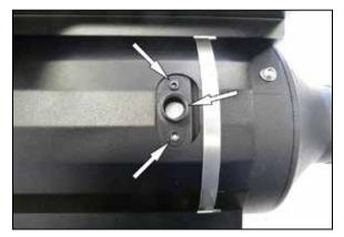
11. Position the drain bracket through the opening in the bracket as shown and use a silver marker or equivalent to mark hole locations to be drilled. Two holes will be for the bolts to hold the drain plate on and the third hole will be a drain hole.
