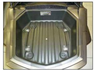
32. Reinstall the cargo box and secure with the factory hardware.
