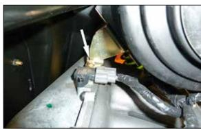
9. Remove the two bolts that secure the air filter housing to the intake manifold using a T30 torx. **NOTE: Access to these bolts is tight.**
