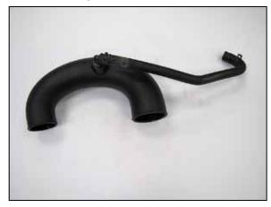
21. Remove the vent fitting from the factory intake tube and install it onto the fitting installed into the  $K\&N^{\mbox{\tiny B}}$  intake tube as shown.
