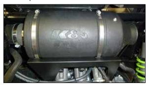
26. Slide the K&N<sup>®</sup> air filter housing onto the bracket and position so the duck bill drain is through the bracket. Secure the air filter housing with the hose clamps.
