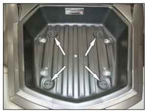
2. Remove the four bolts that secure the cargo tub and then remove the tub from the vehicle.
