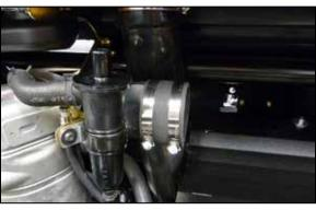
25. Install the provided coupler (08711) onto the K&N<sup>®</sup> intake tube and secure with the provided hose clamp.
