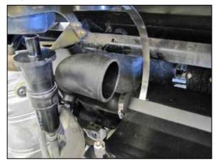
23. Install the K&N® intake tube into the coupler on
