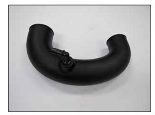
20. Install the vent fitting into the K&N<sup>®</sup> intake tube as shown.
