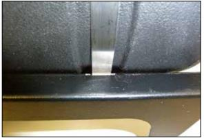
10. Install the K&N<sup>®</sup> air filter housing lid onto the K&N<sup>®</sup> air filter housing without the K&N<sup>®</sup> air filter. Then install the housing onto the mounting bracket and secure with the provided hose clamps as shown.
