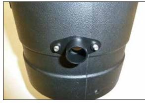
12. Drill two  $\frac{1}{4}$ "id holes for the bolts and one 5/8"id hole for the drain where marked and then secure the drain bracket onto the filter housing.
