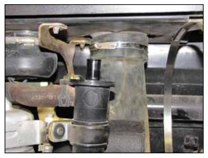
24. Reinstall the clutch fresh air intake hose onto intake and secure with the provided hose clamp.
