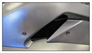
30. Secure the duct to the exterior panel using the provided hardware.
