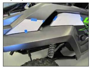
28. Cut out the two drill templates and then tape them to the side panel as shown. Drill 1/4" holes through the panel using the templates as a guide. **NOTE: Align the templates along the bottom edge of the panel.**
