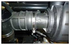
7. Loosen the hose clamp the secures the intake tube to the air filter housing and then disconnect the hose from air filter housing.
