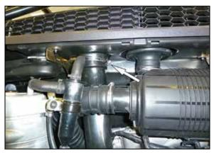
4. Loosen the hose clamp that secures the clutch cover fresh air intake hose to the inlet.
