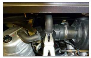
6. Release the spring clamp that secures the breather hose and then disconnect the breather hose.
